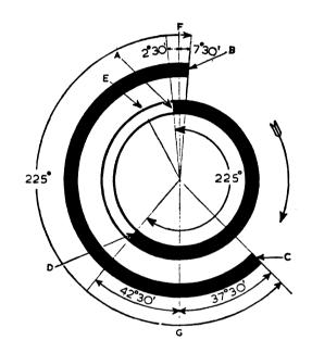
Valve timing diagram—Engine type Six-346
