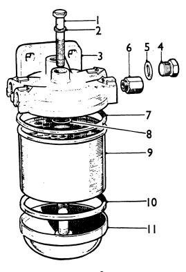
Fig. 3 Main fuel filter components
