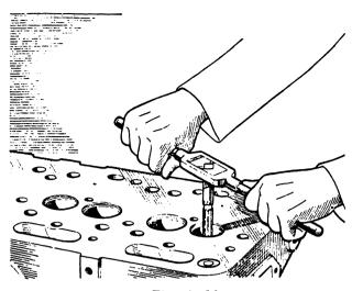
Fig. Aa.16 Reaming a valve guide using tool 18G 229A
