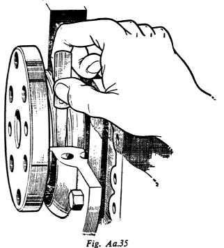
Checking the crankshaft rear oil seal cover to oil return thread clearance
