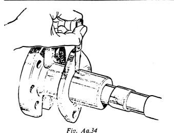
Checking the camshaft end-float
