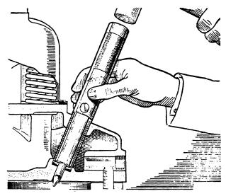
Fig. Aa.20 Installing an injector sleeve, using tool 18G 561
