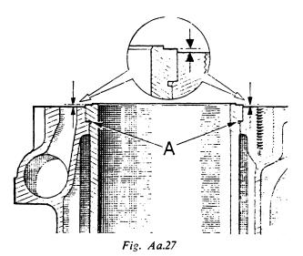
Insert shims at (A) to adjust the standing height of the early cylinder liner. Shown inset are the faces of the cylinder block and the liner from which the standing height is measured
