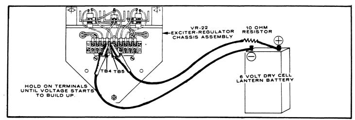
FIGURE 7. FLASHING THE FIELD
