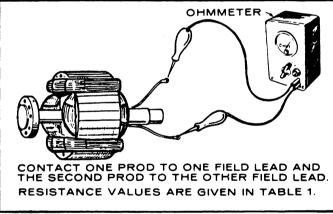
FIGURE 19. TESTING ROTOR FOR AN OPEN CIRCUIT
