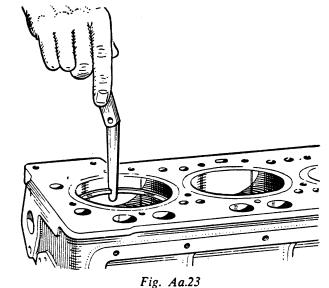
When checking the gap clearance of a new piston ring ensure that the ring is inserted into an unworn part of the cylinder bore
