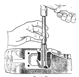
Fig. Aa.15 Driving a valve guide into position, using tool 18G 228
