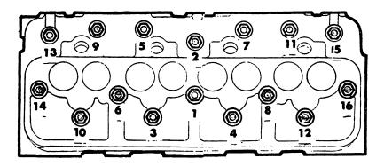
Fig. Aa. 8B (SIX-346) Cylinder head nut slackening and tightening sequence
