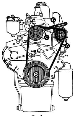
Fig. 5 Fan belt adjustment
