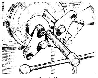
Fig. Aa.29 Withdrawing the crankshaft pulley, using tools 18G 231 and 18G 231 A
