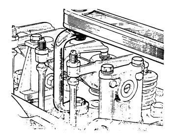
Fig. Aa.9 Using spanner 18G 396 and torque wrench 18G 372 to tighten the cylinder head nuts
