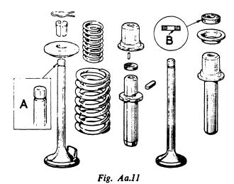
Engine value components showing the locating flat (A) on the inlet value and the chamfered bore (B) of the exhaust value oil seal
