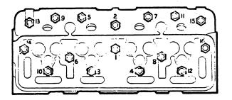
Fig. Aa. 8A (FOUR-230) Cylinder head nut slackening and tightening sequence
