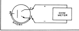
Checking Unijunction Transistors (shown on regulator diagram as Q3):
