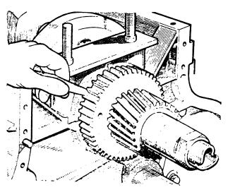
Fig. Aa.37 Checking the crankshaft end-float
