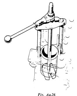
Withdrawing a cylinder liner, using tool 18G 227 C
