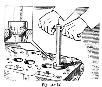
Badly pitted valve seats should be refaced, using tools 18G 27, 18G 28, 18G 28 A, 18G 28 B, 18G 28 C, 18G 174, 18G 174 A, 18G 174 B, 18G 174 C, and 18G 230
