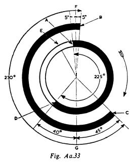
Valve timing diagram Four-230
