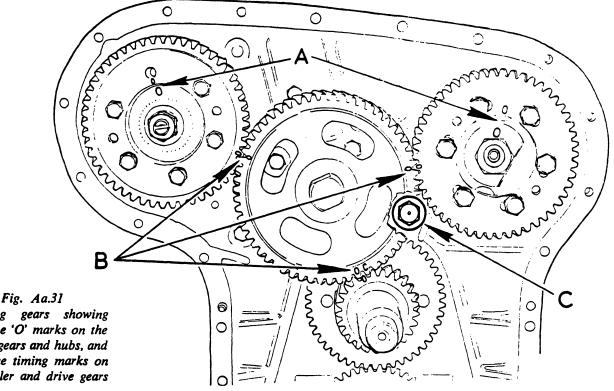
Timing gears showing (A) the 'O' marks on the drive gears and hubs, and (B) the timing marks on the idler and drive gears
