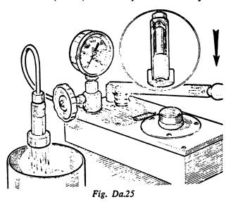
Reverse flushing an injector nozzle, using testing machine 18G 109 A and adaptor 18G 109 E. Shown inset is a sectioned adaptor with the nozzle in position.
