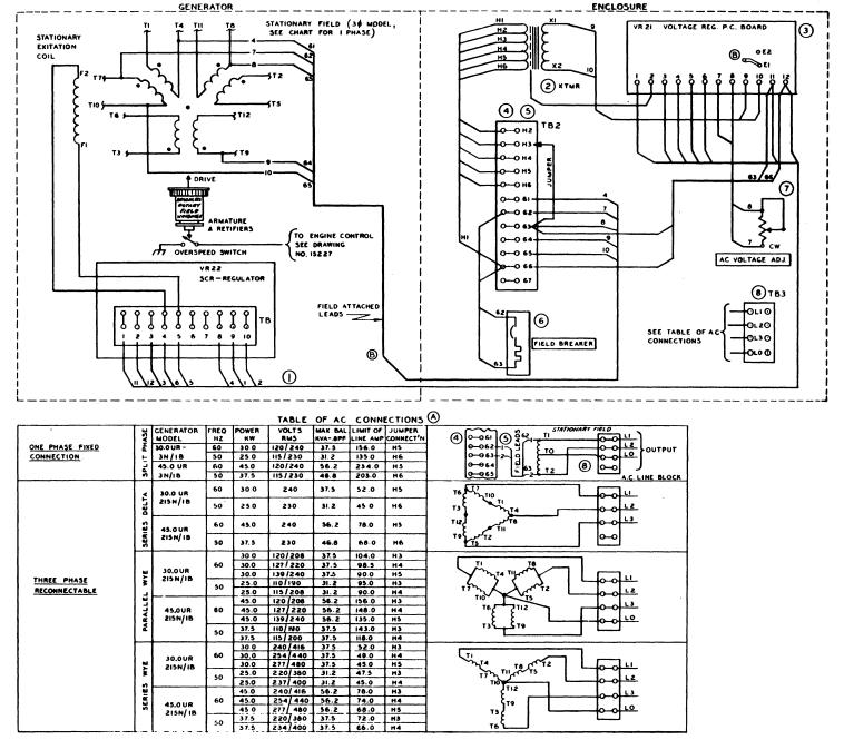
& 45KW: VOLTAGE REGULATOR & POWER CONNECTIONS
