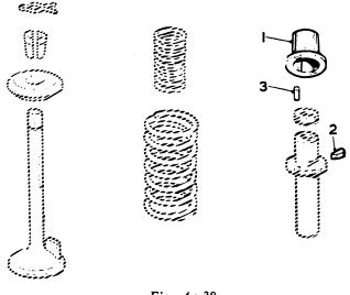
Fig. Aa.38 Modified inlet valve locating details 1 Thimble. 2 Key. 3 Dowel.
