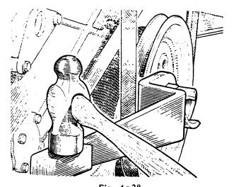
Fig. Aa.28 Removing the starting handle jaw nut, using tool 18G 97
