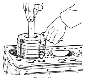
Fig. Aa.21 Installing a piston and connecting rod assembly using tool 18G 55 A
