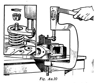
Compressing the valve springs, using tool 18G 106
