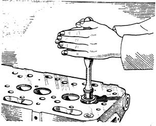
Fig. Aa.13 Grinding-in a valve, using tool 18G 29
