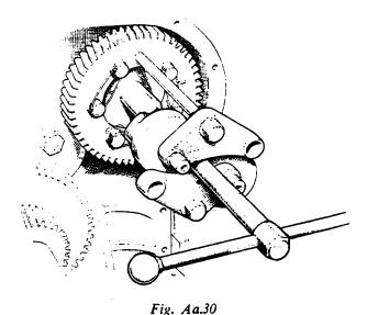
Withdrawing the camshaft gear, using tools 18G 231, 18G 231 C, and 18G 231 D
