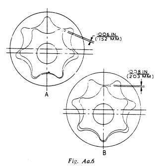
Check the oil pump rotor lobe clearance with the rotors in positions A and B. The dimensions given are for the maximum clearance
