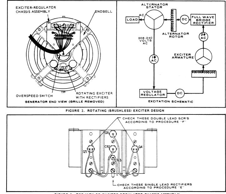
FIGURE 3. TOP VIEW OF EXCITER-REGULATOR CHASSIS ASSEMBLY
