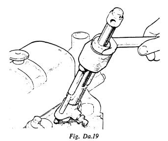
Withdrawing an injector, using tool 18G 491 A
