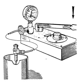
Fig. Da.27 An injector assembled to machine 18G 109 A ready for spray testing
